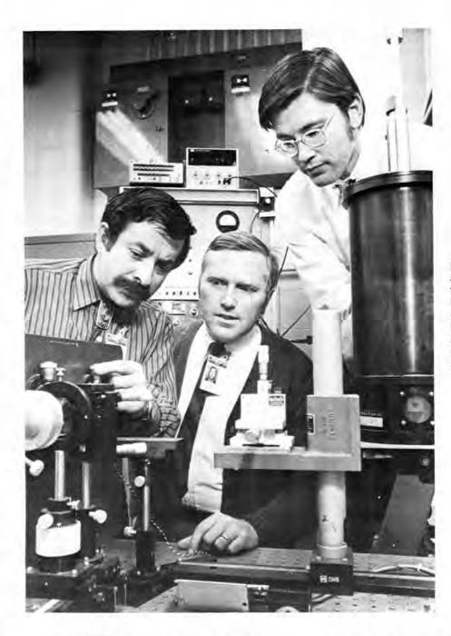
KEN TOURYAN (5640, lett) adjusts the entrance slit on a tunable diode laser as Colin Hackett and Dave Smith (both 5642) look on. The laser would be a primary analytical tool of a stratospheric measurement program.
